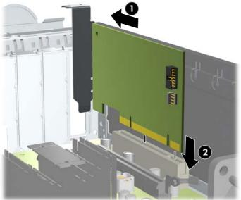
Figure 6-21 Installing an Expansion Card
